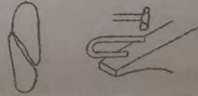
Fig. 5 - Scarfing ends of link with ball peen hammer.
